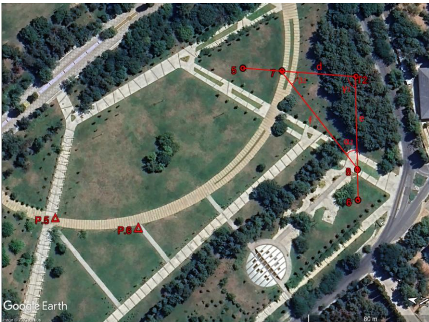
Figure 4: Map of the second test area with an angle value of approximately 100g ( 105g in the study).
